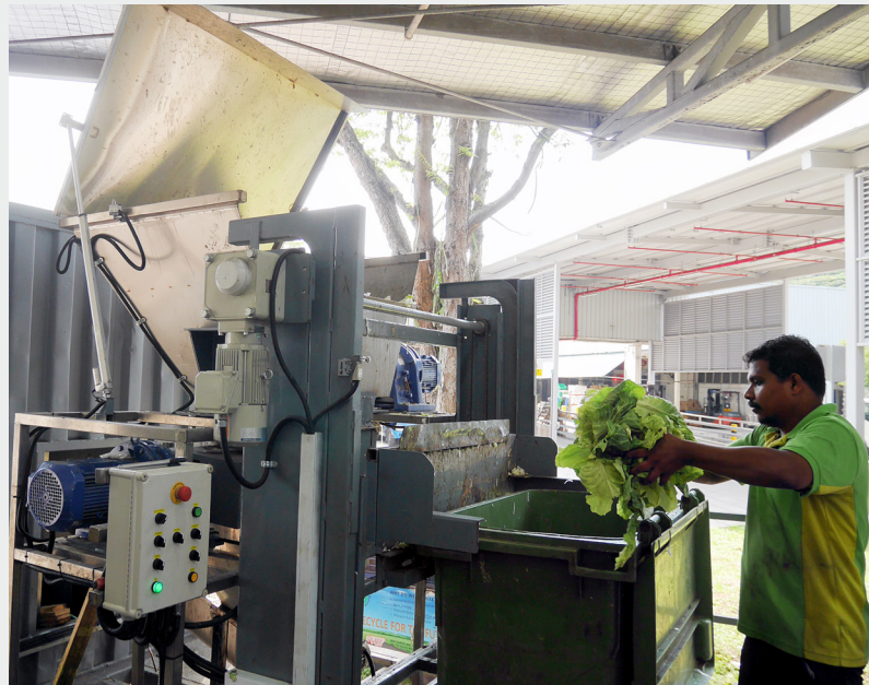
Food and horticulture waste is converted into compost through a food waste digester at Pasir Panjang Wholesale Centre
