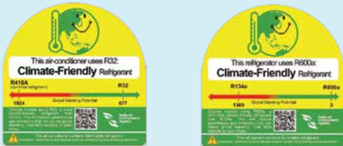
The Voluntary Labels for air-conditioners (left) and refrigerators (right) using climate-friendly refrigerants
